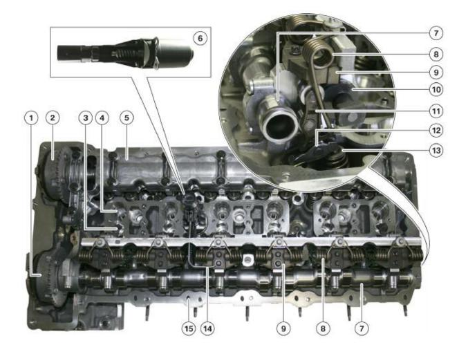
Note: Notice the hollow, lightweight design of the camshafts (7) and the blow-by passages leading into the intake ports (15).
